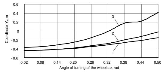
Fig. 5. Dependence of coordinate  $Y_a$  on turning angle  $\alpha$  of driven wheels of tractor at various speeds of their movement on turning strip  $V_i$ :  $1 - 1.0 \text{ m} \cdot \text{s}^{-1}$ ;  $2 - 2.0 \text{ m} \cdot \text{s}^{-1}$ ;  $3 - 3 \text{ m} \cdot \text{s}^{-1}$
