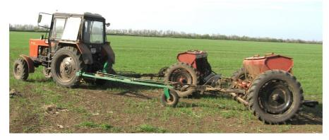
Fig. 1. Experimental two-machine sowing aggregate moving on turn
