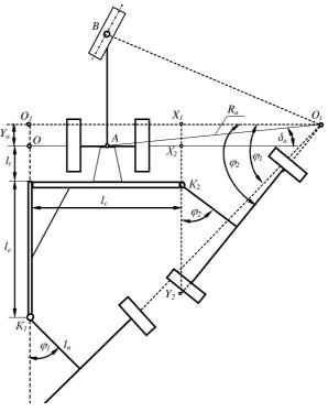
Fig. 3. Scheme for determination of turning angles of trailed seeders
