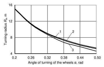
Fig. 4. Dependence of turning radius  $R_a$  of sowing aggregate on turning angle  $\alpha$  of driven wheels of tractor at various speeds of movement on turning strip  $V_t$ :  $1 - 1.0 \text{ m} \cdot \text{s}^{-1}$ ;  $2 - 2.0 \text{ m} \cdot \text{s}^{-1}$ ;  $3 - 3 \text{ m} \cdot \text{s}^{-1}$
