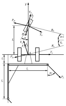
Fig. 2. Equivalent turning scheme of two-machine sowing aggregate
